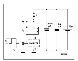
Fig. 3: Switching Times Test Circuits For Resistive Load
