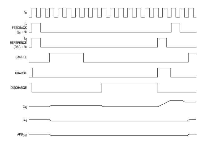
Figure 13. Timing Diagram for Minimum Divide Value (N = 16)
