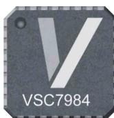
The VSC7984 is a 11.3Gb/s clocked modulator driver for SONET/SDH and 10GbE applications. The device provides selectable data retiming to improve jitter performance and controls for output bias voltage, modulation voltage, and duty cycle. Internal operational amplifiers and on-chip voltage
