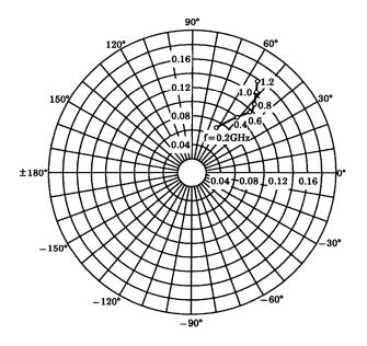
$\begin{array}{c} S_{21e} \\ V_{CE} = 10V \\ I_{C} = 2mA \\ Ta = 25^{\circ}C \end{array}$
