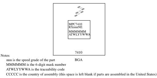
Figure 26. Freescale Part Marking for BGA Device
