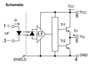
0.1  $\mu$ F bypass capacitor must be connected between pins 6 and 4. (Note 4) Unit in mm
