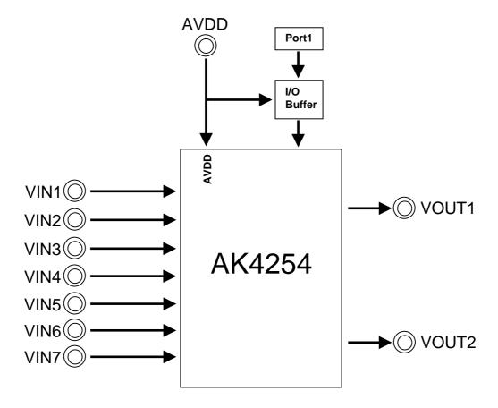
Figure 1. AKD4254-A Block Diagram
