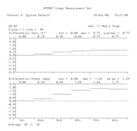
Figure 1-4 DG, DP (Input= Modulated 5 Step)
