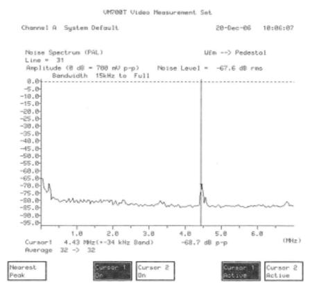
Figure 1-3 Crosstalk (Input= 100% red Y-Signal (VIN2), measured at VOUT1)
