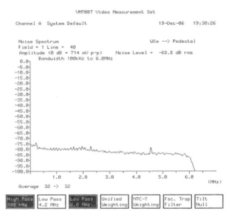
Figure 1-1. Noise spectrum (Input=0%flat field, BW=100kHz to 6MHz)
