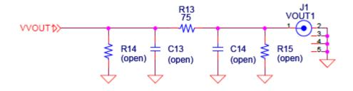
Figure 4. VOUT1 Output circuit
