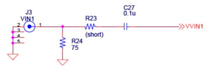
Figure 3. VIN Input circuit
