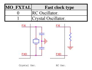
The RC oscillator has a built-in capacitor. An external resistor is needed to connect from FXI to GND to determine the oscillation frequency. The capacitance of internal RC oscillator is selected by mask option MO\_RCAP[2..0].
