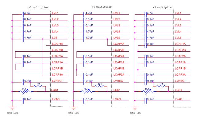
Different duties require different bias settings. There is some theoretical correspondence between the Duty and Bias Setting. However, it is better to use it as starting point and adjust it with real LCD panel connected to it to determine the final setting. The theoretic relationship between the duty and bias setting as following:
