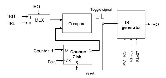
To avoid unexpected IR output, users should firstly load the content of IRH and IRL before turn on IR by set IROE bits to '1'.
