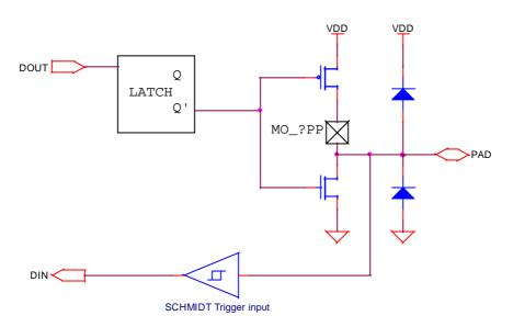
As pads of PRT15 and PRT17 are shared with LCD segment driver, the function of the pad is determined by mask options. Following table is the setting for MO\_LIO?[...] and MO\_?PP[...] and others related to LCD display setting and pin assignment features.
