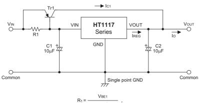
$$R_1 = \frac{V_{BE1}}{I_{REG} - \frac{I_{C1}}{(1+\beta)}}$$
