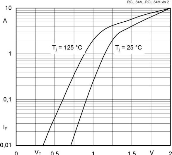
Fig. 1 Forward characteristics ( typical values )
