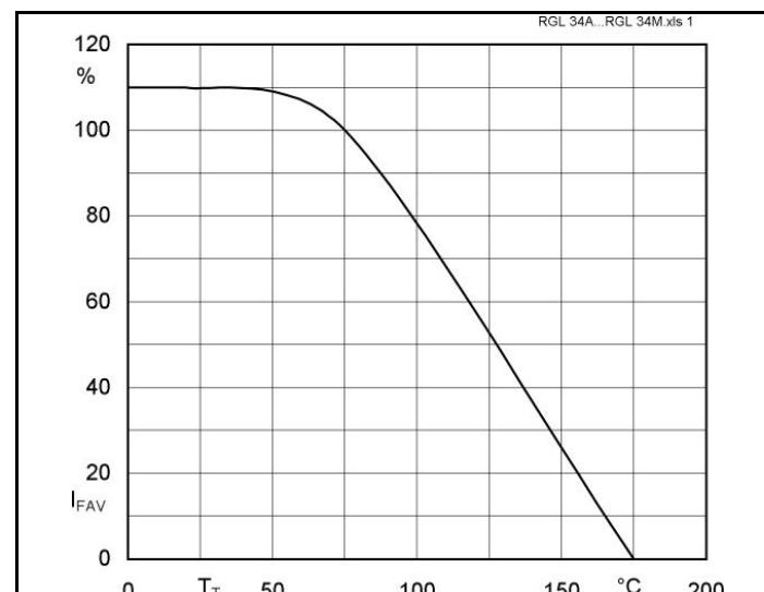
Fig. 2 Rated forward current vs. temp. of the terminals <sup>4)</sup>
