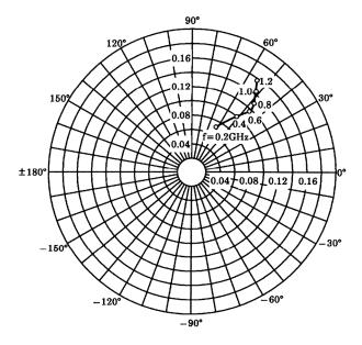
$\begin{array}{l} S_{21e} \\ V_{CE} = 10V \\ I_{C} = 2mA \\ Ta = 25^{\circ}C \end{array}$
