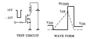
$$\begin{array}{ll} R_G\!=\!25\Omega \\ V_{DD}\!=\!-50V,\; L\!=\!10.5mH \end{array} \quad E_{AS}\!=\!\frac{1}{2}\cdot L\cdot I^2\cdot (\frac{B_{VDSS}}{B_{VDSS}\!-\!V_{DD}})$$
