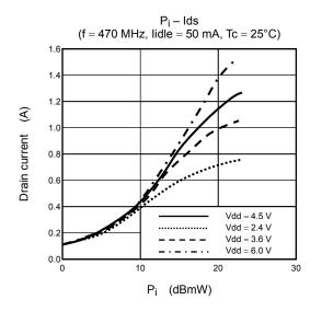
Caution: These are typical curves and devices are not necessarily guaranteed at these curves.
