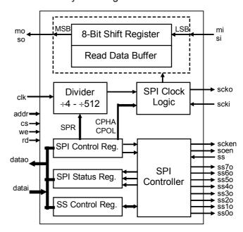
**Control Register** may be read or written at any time, is used to configure the DSPI System. This register controls the mode of transmission (Master, Slave), polarity and phase of SPI Clock and transmission speed.
