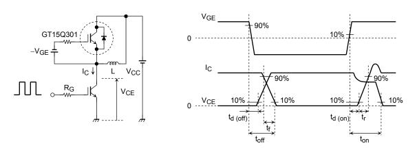
Note2: Switching loss measurement waveforms
