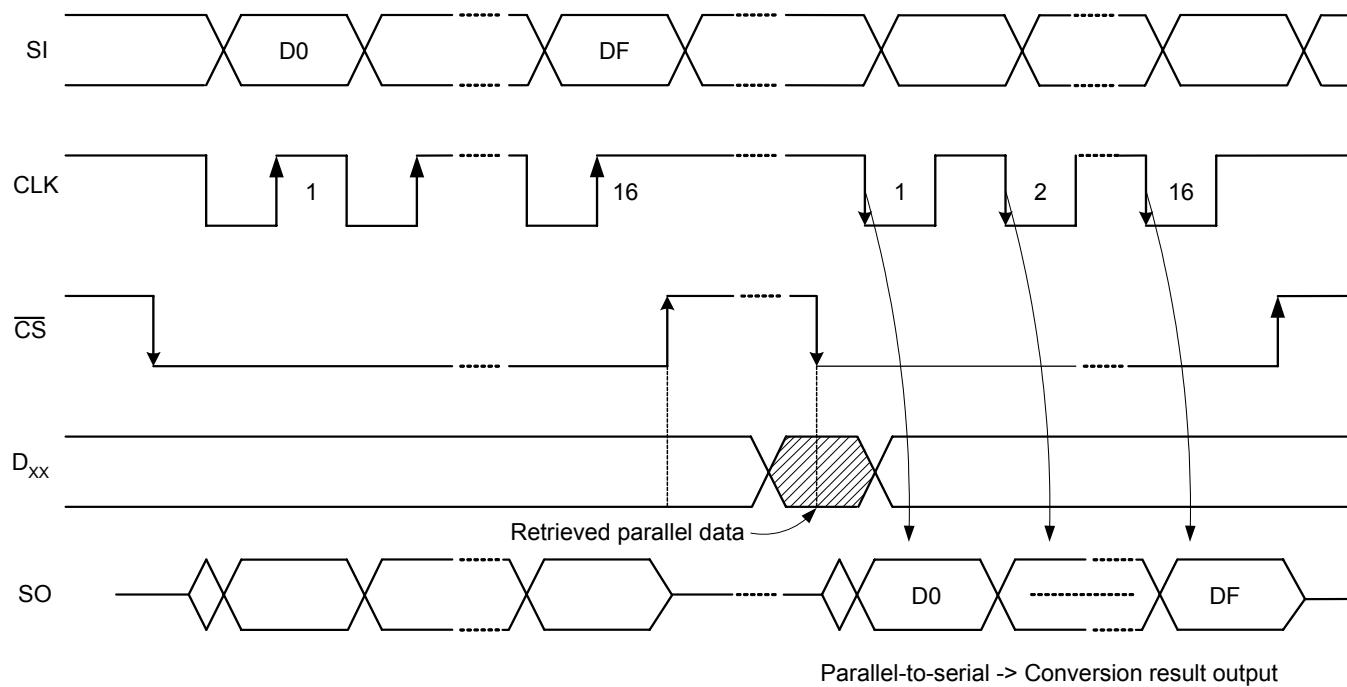
Data input is enabled at the falling edge of the /CS signal. 16-bit data (parallel → serial conversion commands) is input and commands accepted at the rising edge of /CS. AT the falling edge of /CS, data from the parallel input is loaded into bits D4 to DF of the shift register, and output from the SO pin timed to the falling edge of the CLK signal.
