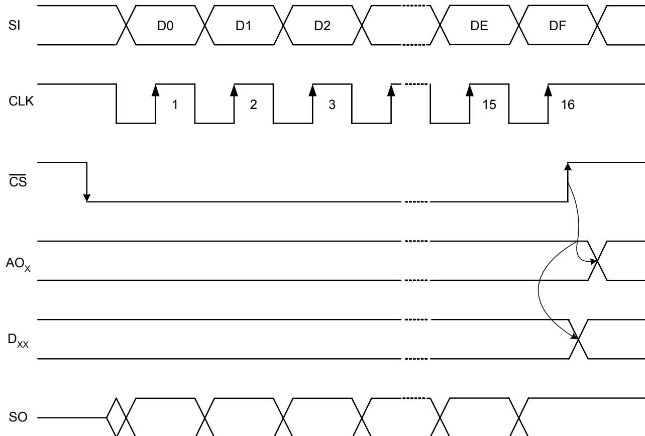
Data input is enabled at the falling edge of the /CS signal. 16-bit data is input, and the shift register command is executed at the rising edge of /CS.
