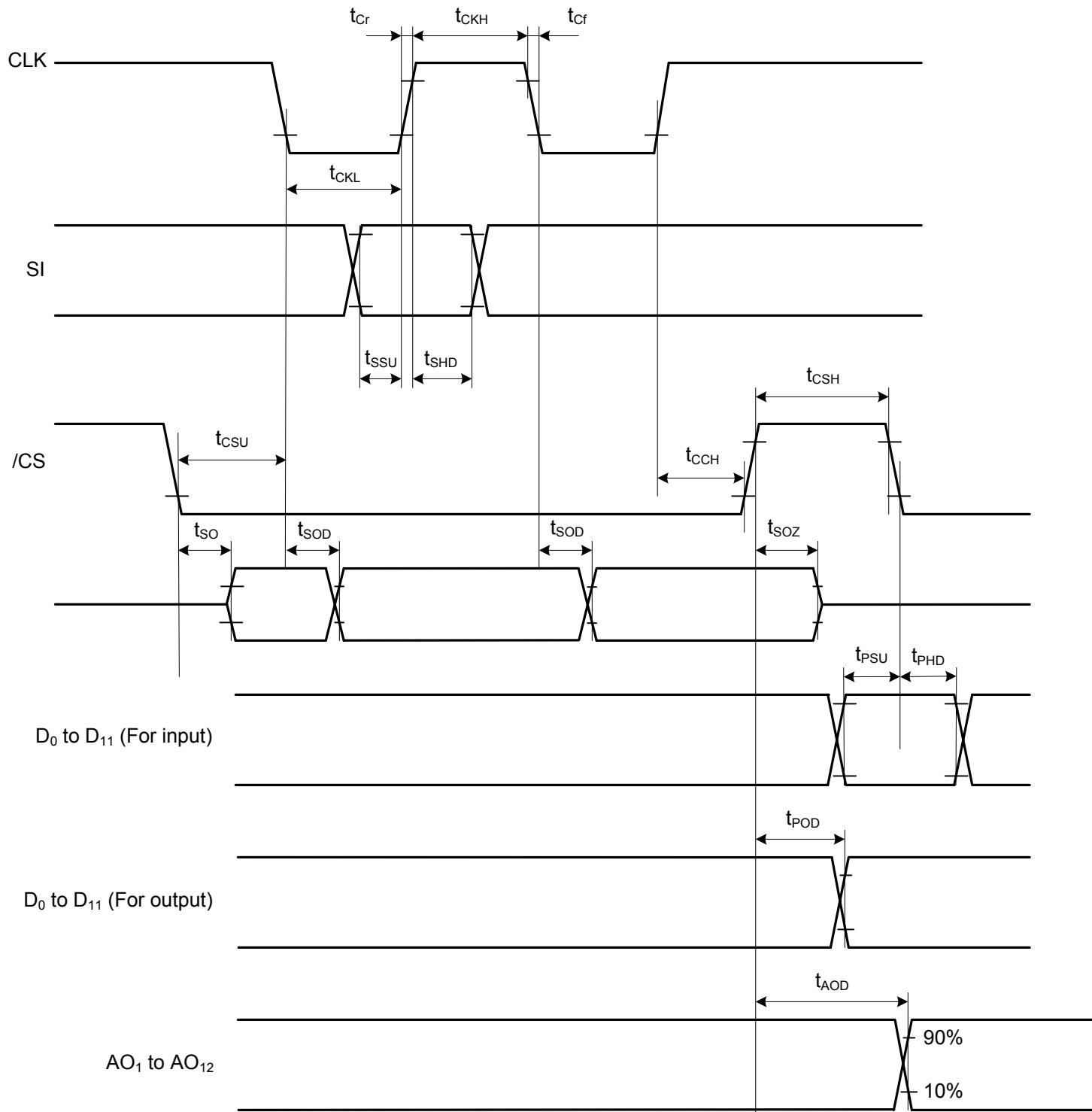
The decision level for CLK, SI, /CS, SO, and D<sub>0</sub> to D<sub>3</sub> is 80% and 20% of VCCD. The decision level for D<sub>4</sub> to D<sub>11</sub> is 80% and 20% of VCCA, and for AO<sub>1</sub> to AO<sub>12</sub> is 90% and 10% of VCCA.
