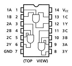
Japan TC74AC11P DIP14-P-300-2.54 TC74AC11F SOP14-P-300-1.27A TC74AC11FN SOL14-P-150-1.27 Weight DIP14-P-300-2.54 : 0.96 g (typ.) SOP14-P-300-1.27A : 0.18 g (typ.) SOL14-P-150-1.27 : 0.12 g (typ.)
