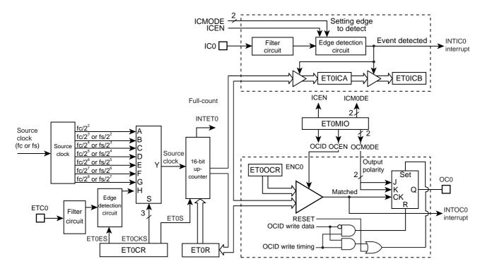
Figure 8-1 Extended Timer-Counter 0 (ETC0)
