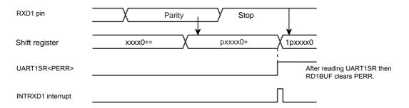
Figure 12-5 Generation of Parity Error
