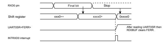
Figure 11-6 Generation of Framing Error
