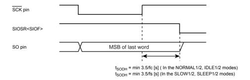
Figure 10-9 Transmiiied Data Hold Time at End of Transfer
