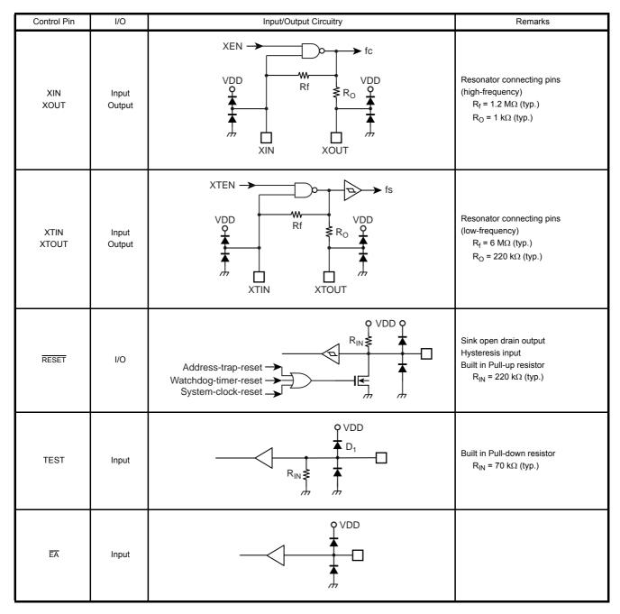
Note: The TMP86PH06 does not have a pull-down resistor (R<sub>IN</sub>) and a diode (D<sub>1</sub>) for TEST pin. Be sure to fix the TEST pin to low level in MCU mode.
