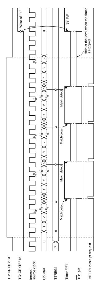
Figure 9-4 8-Bit PDO Mode Timing Chart (TC1)
