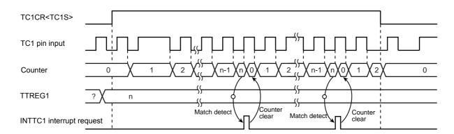
Figure 9-3 8-Bit Event Counter Mode Timing Chart (TC1)
