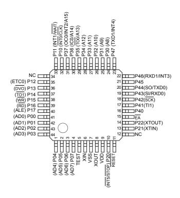
Figure 1-1 Pin Assignment
