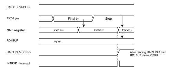
Figure 12-7 Generation of Overrun Error
