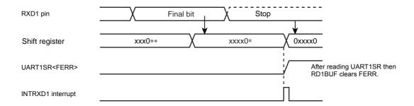
Figure 12-6 Generation of Framing Error
