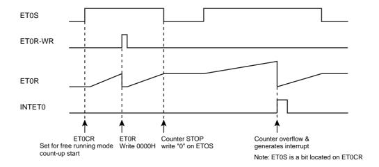
Figure 8-2 Example for Free-running mode operation
