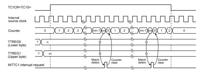
Figure 9-6 16-Bit Timer Mode Timing Chart (TC0 and TC1)
