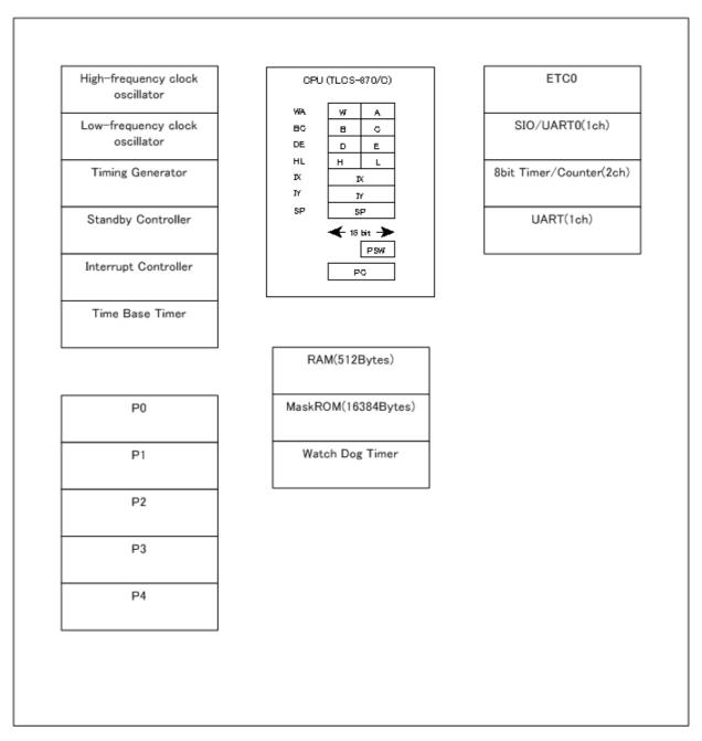
Figure 1-2 Block Diagram
