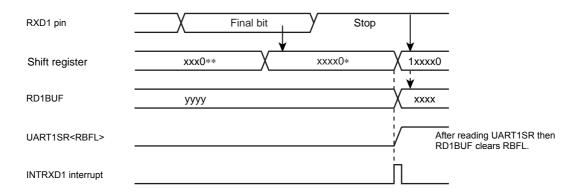
Figure 12-8 Generation of Receive Data Buffer Full
