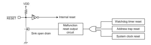
Figure 2-15 Reset Circuit
