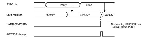
Figure 11-5 Generation of Parity Error
