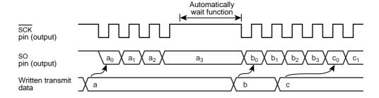
Figure 10-3 Automatic Wait Function (at 4-bit transmit mode)
