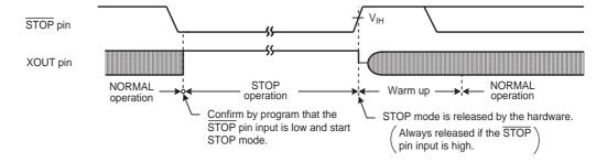
Figure 2-7 Level-sensitive Release Mode
