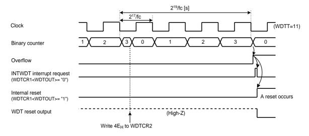
Figure 6-2 Watchdog Timer Interrupt/Reset
