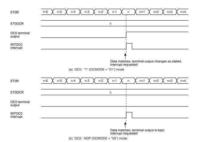
Figure 8-6 Examples for comparing operation
