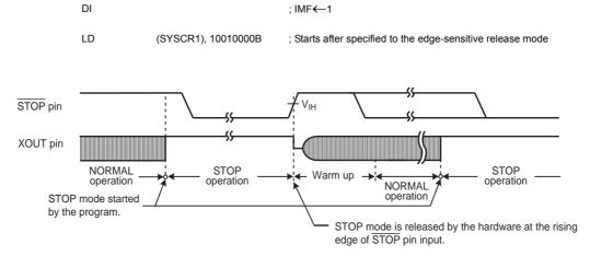
Figure 2-8 Edge-sensitive Release Mode
