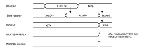
Figure 11-8 Generation of Receive Data Buffer Full
