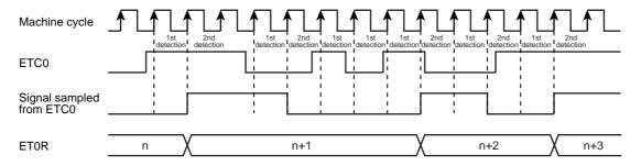
Figure 8-3 Edge Filtering in Event Counter Mode (Rising Edge Detection)
