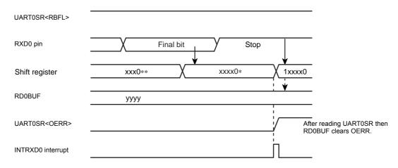
Figure 11-7 Generation of Overrun Error
