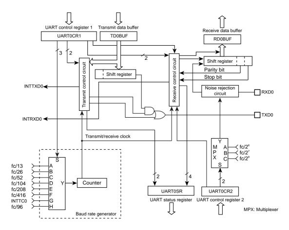
Figure 11-1 UART0 (Asynchronous Serial Interface)
