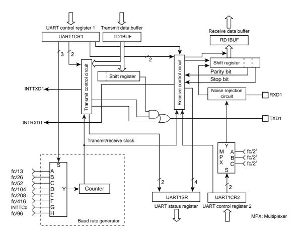
Figure 12-1 UART1 (Asynchronous Serial Interface)
