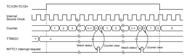
Figure 9-2 8-Bit Timer Mode Timing Chart (TC1)
