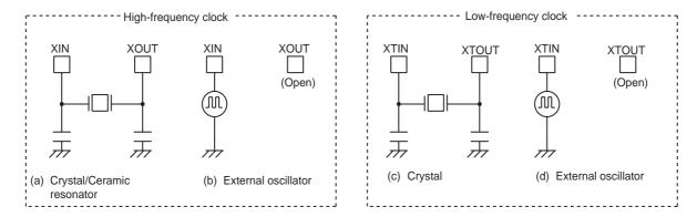
Figure 2-3 Examples of Resonator Connection
