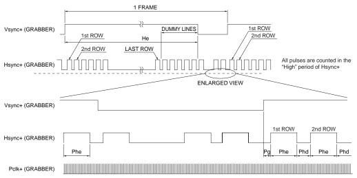
All pulses are counted at the riging edge of Pclk+. The effective video output is only included in the "Phe" period.
