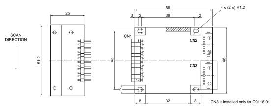
Component mounting height: 3.6 mm
