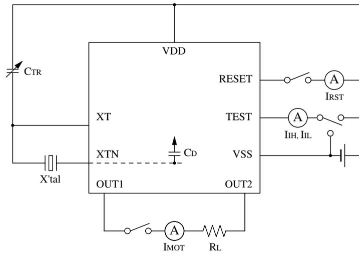
X'tal parameters:  $f = 32.768\text{kHz}$ ,  $C_1 = 20\text{k}\Omega$ ,  $C_0 = 1.3\text{pF}$ ,  $C_1 = 2.6\text{fF}$
