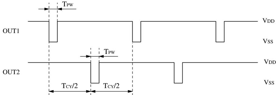
Watch movement period  $T_{cy} = 2s$ , Pulsewidth  $T_{pw} = 3.9ms$
