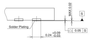
Note:Cutting burr of lead are 0.05mm MAX.
