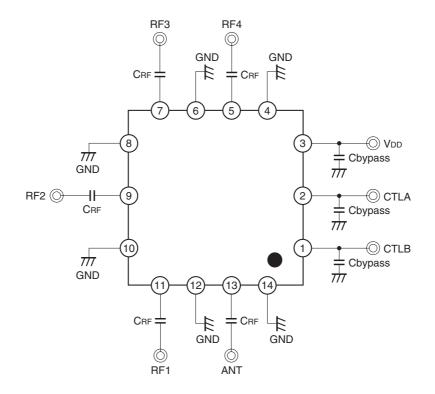
When using this IC, the following external components should be used: CRF: This capacitor is used for RF decoupling and must be used for all applications. Cbypass: This capacitor is used for DC line filtering. 100pF is recommended.
