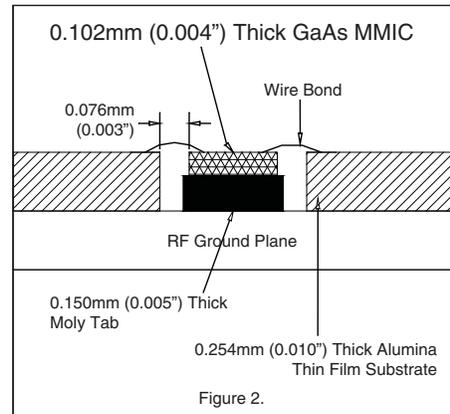
**General Handling:** Handle the chip along the edges with a vacuum collet or with a sharp pair of bent tweezers. The surface of the chip has fragile air bridges and should not be touched with vacuum collet, tweezers, or fingers.
