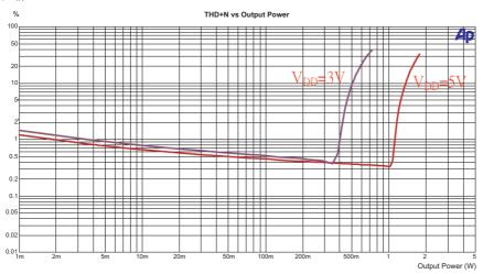
•  $R_{LOAD}$ =8 $\Omega$ ,  $V_{IN}$ =1kHz sinewave
