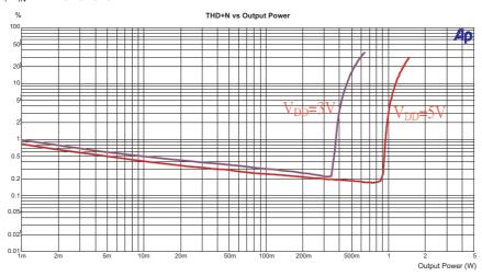
•  $R_{LOAD}$ =16 $\Omega$ ,  $V_{IN}$ =1kHz sinewave
