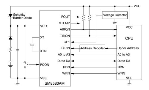
Note. Because all the circuit components, except the crystal unit, are built in the SM8580AM chip, the oscillation circuit is realized just by the connection of the 32.768kHz crystal unit between XT and XTN terminals. The digital correction function is used to adjust the accuracy of clock time.
