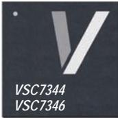
Barrington-II (VSC7344) is an advanced Ethernet MAC containing 24 10/100/1000 Ethernet ports with integrated SGMII and 100/1000 optical serializers/deserializers. The host interface can be configured as SPI-4.2, one XAUI, or two XAUI interfaces. Each SPI-4.2 and XAUI host interface uses a SPI-4.2 status channel for flow control. To support the high oversubscription factor, the Barrington-II has a set of advanced QoS features.
