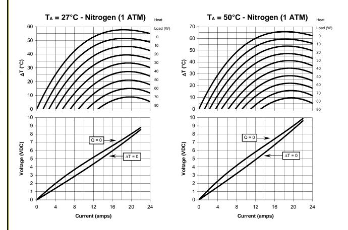
For performance information in a vacuum or with hot side temperatures other than  $27^{\circ}\text{C}$  or  $50^{\circ}\text{C}$ , consult one of our Applications Engineers.
