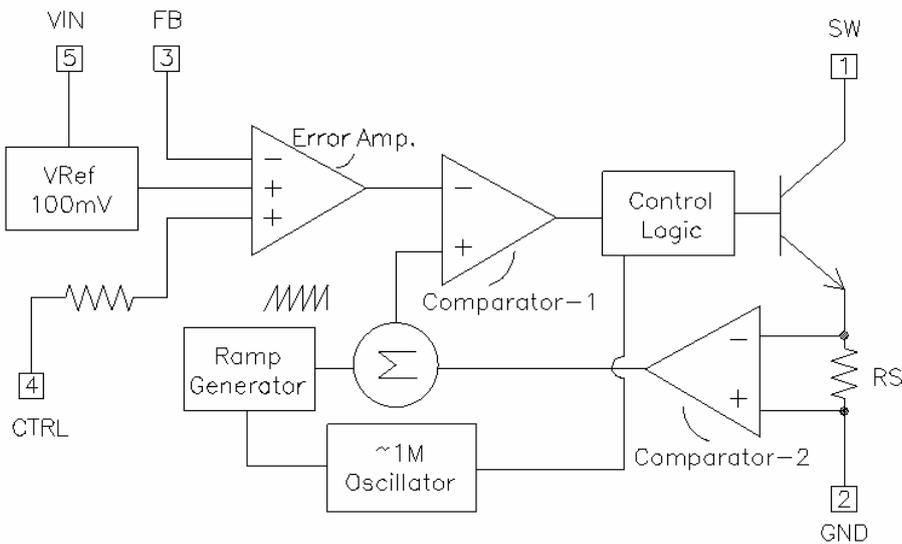
**Figure 3: YB1517 Block Diagram**
