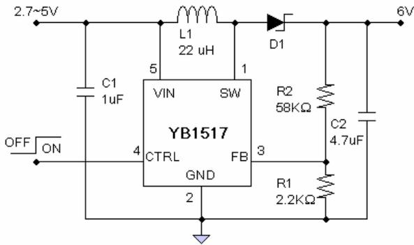
Figure 5 : TFT Panel Power Application Circuit
