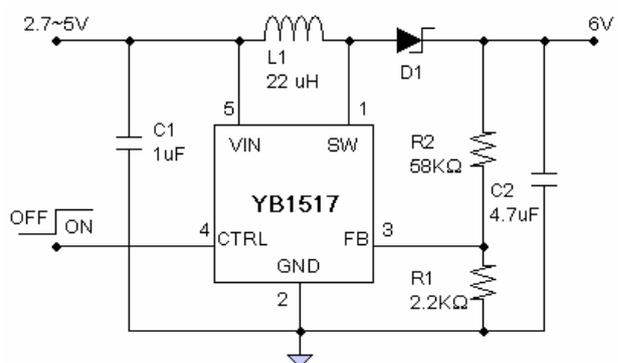
Figure 2 : DC-to-DC Converter
