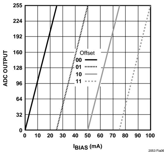
Figure 6. Quarter Scale (code 01<sub>BIN</sub>) with Offset
