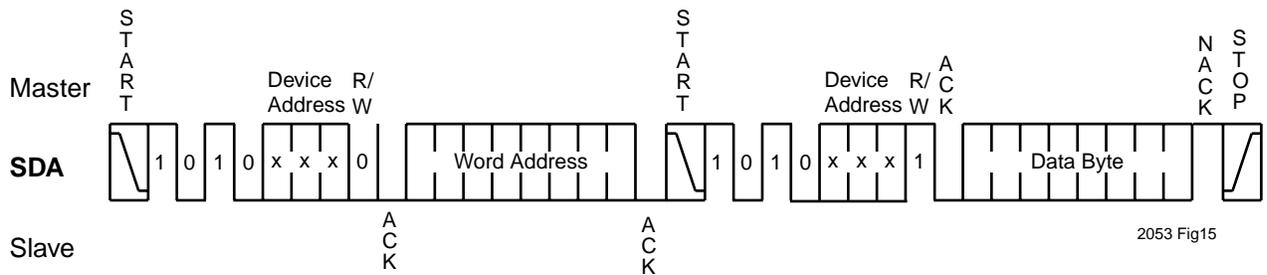
Figure 15. Look-up Table Random Address Read with Dummy Write
