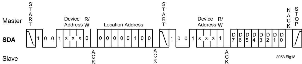
Figure 18. 8-Bit DAC Volatile Register Read with Dummy Write
