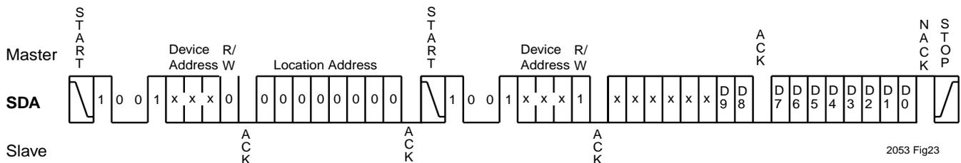
Figure 23. 10-Bit DAC Volatile Register Read with Dummy Write
