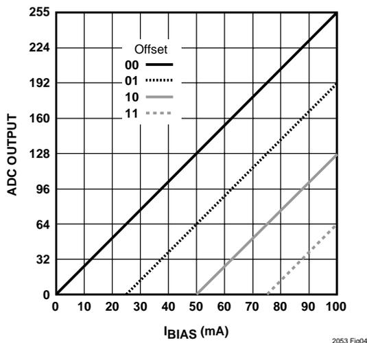
Figure 4. Full Scale (code 11<sub>BIN</sub>) with Offset
