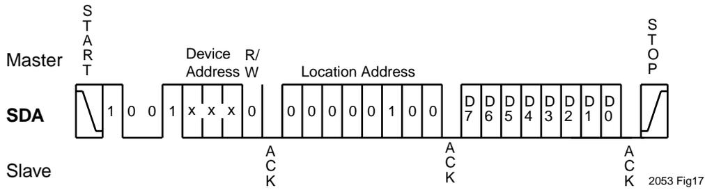
Figure 17. 8-Bit DAC Volatile Register Write
