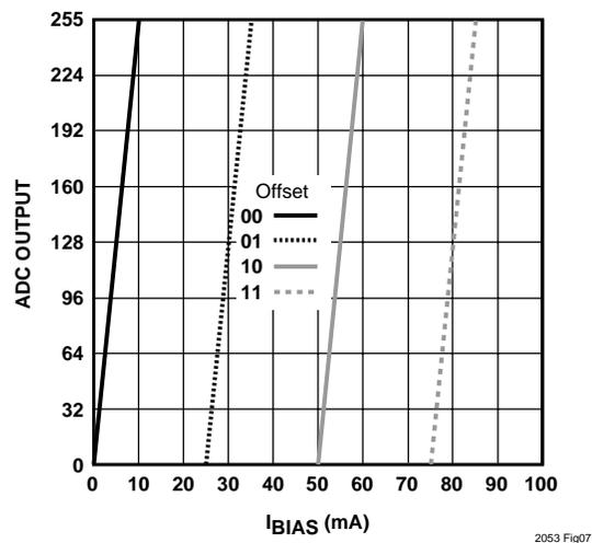
Figure 7. Tenth Scale (code 00<sub>BIN</sub>) with Offset
