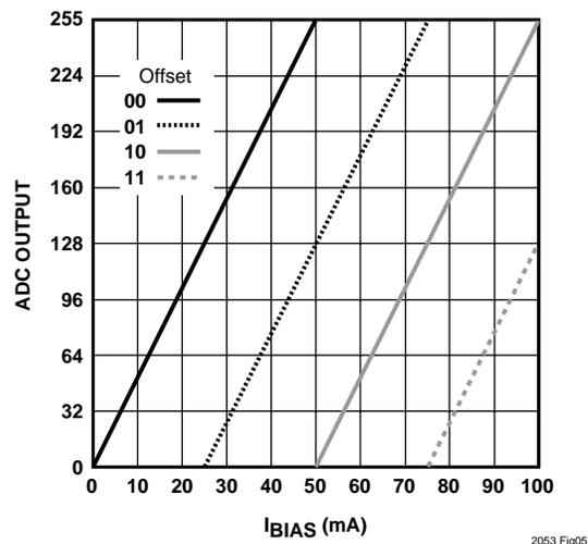
Figure 5. Half Scale (code 10<sub>BIN</sub>) with Offset
