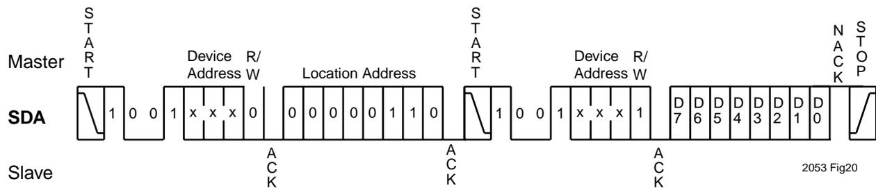
Figure 20. 8-Bit DAC Non-volatile Register Read with Dummy Write
