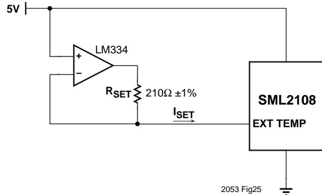
Figure 25. Example of an External Temperature Sensing Device
