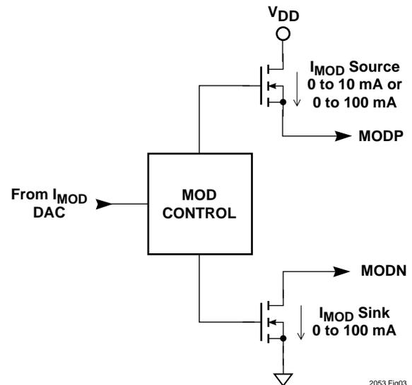
Figure 3. Output Block 2: I<sub>MOD</sub>
