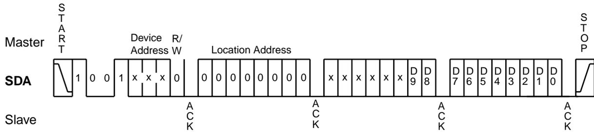
Figure 21. 10-Bit DAC Volatile Register Write
