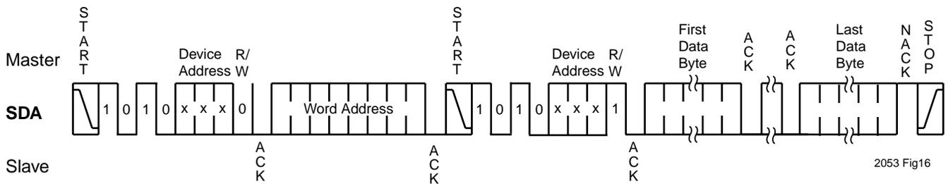
Figure 16. Look-up Table Sequential Read with Dummy Write
