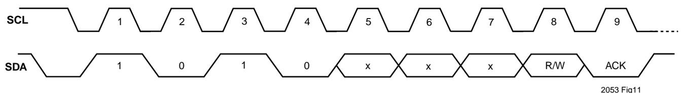
Figure 11. Typical Master Address Byte Transmission
