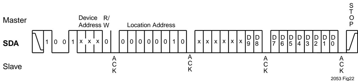
Figure 22. 10-Bit DAC Nonvolatile Register Write
