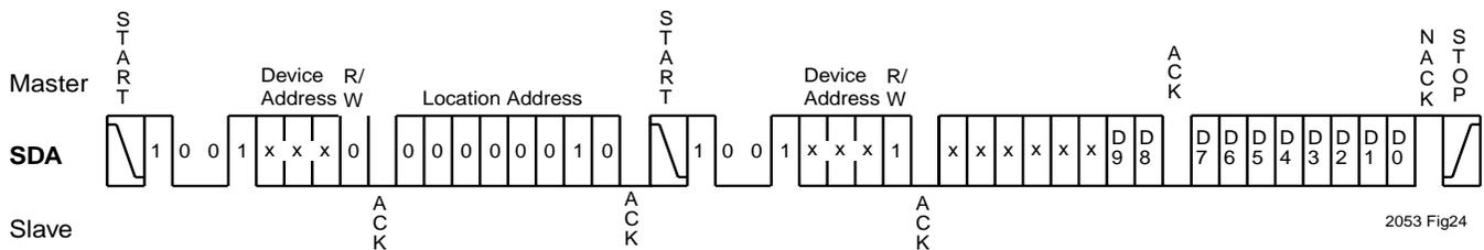
Figure 24. 10-Bit DAC Nonvolatile Register Read with Dummy Write
