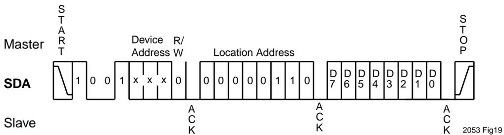
Figure 19. 8-Bit DAC Non-volatile Register Write
