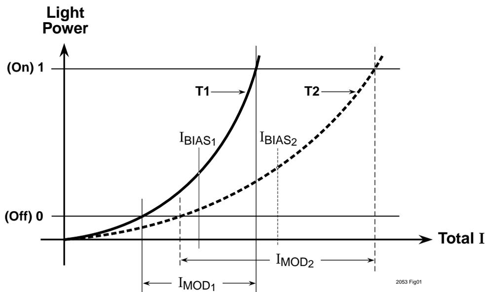
Figure 1. Laser Current Increase Caused by Temperature Increase, Constant Light Power Out
