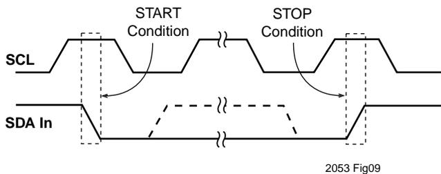
Figure 9. I<sup>2</sup>C Start and Stop Timing
