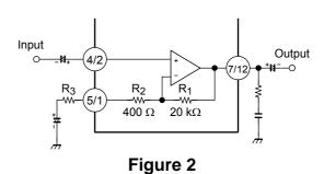
To shiba has confirmed that the  $G_V$  (min) is approximately 28 (dB) on a regular printed circuit board. However, if the value of  $R_2 + R_3$  is larger, the feedback voltage increases and oscillation will start. Determine the value of  $R_2 + R_3$  to ensure proper startup behavior under actual usage conditions.
