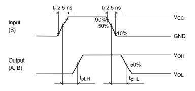
Figure 2 t<sub>pLH</sub>, t<sub>pHL</sub>
