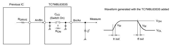
R<sub>DRIVE</sub> = output impedance of the previous IC
