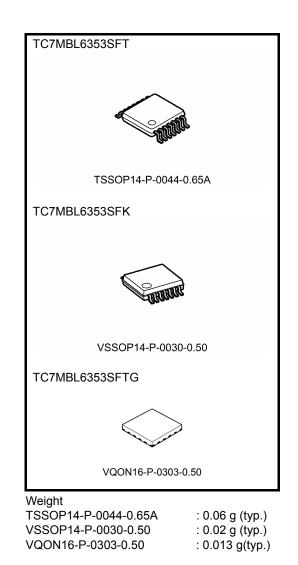
Note: When mounting VQON package, the type of recommended flux is RA or RMA.
