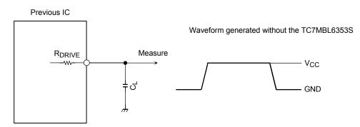
R<sub>DRIVE</sub> = output impedance of the previous IC
