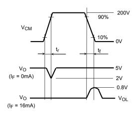
$$CM_H = \frac{160(V)}{t_f(\mu s)}, CM_L = \frac{160(V)}{t_f(\mu s)}$$
