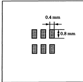
**Figure 1** 25.4 mm × 25.4 mm × 1.6 t, Cu Pad: 0.32 mm<sup>2</sup> × 6
