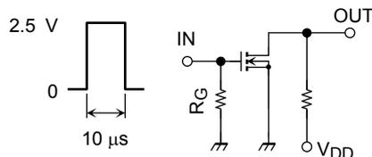
$V_{DD} = 10 V$
