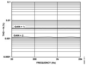
Figure 31. THD+N vs. Frequency,  $V_{OUT} = 10 \text{ V p-p}$
