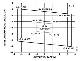
Figure 12. Input Common-Mode Voltage vs. Output Voltage,  $Gain = 2, \pm 5 V \text{ and } \pm 2.5 V \text{ Supplies}$
