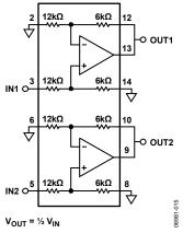
Figure 38. Noninverting Amplifier,  $G = \frac{1}{2}$
