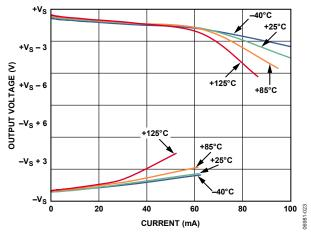
Figure 19. Output Voltage vs. IOUT
