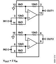
Figure 41. Noninverting Amplifier, G = 3
