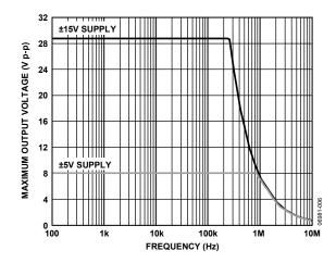
Figure 14. Maximum Output Voltage vs. Frequency
