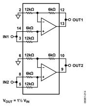
Figure 40. Noninverting Amplifier, G = 1.5
