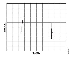
Figure 23. Small Signal Pulse Response for 100 pF Capacitive Load, Gain = ½
