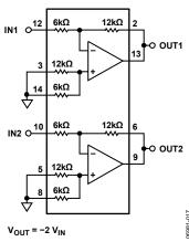
Figure 37. Inverting Amplifier, G = 2
