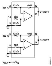
Figure 36. Inverting Amplifier,  $G = \frac{1}{2}$
