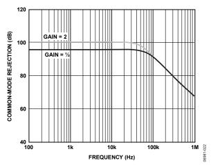
Figure 16. Common-Mode Rejection vs. Frequency, Referred to Input
