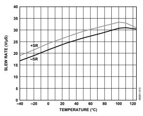
Figure 30.Slew Rate vs. Temperature
