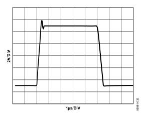
Figure 28. Large Signal Pulse Response Gain =  $\frac{1}{2}$
