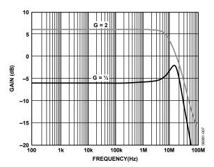
Figure 15. Gain vs. Frequency
