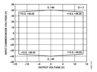
Figure 11. Input Common-Mode Voltage vs. Output Voltage,  $Gain = 2, \pm 15 \text{ V Supplies}$
