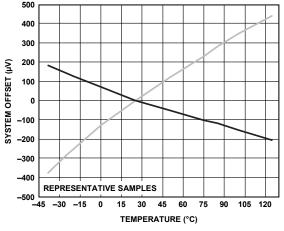
Figure 7. System Offset vs. Temperature, Normalized at 25°C, Referred to Output
