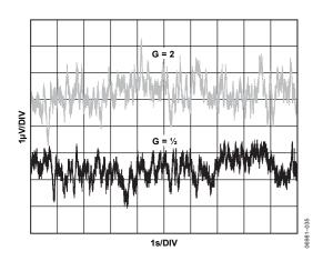
Figure 33. 0.1 Hz to 10 Hz Voltage Noise, RTO
