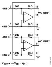
Figure 34. Difference Amplifier,  $G = \frac{1}{2}$
