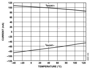
Figure 17. Short-Circuit Current vs. Temperature
