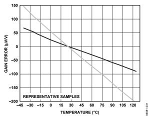
Figure 8. Gain Error vs. Temperature, Normalized at 25°C
