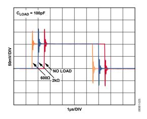
Figure 21. Small Signal Step Response, Gain = 1/2
