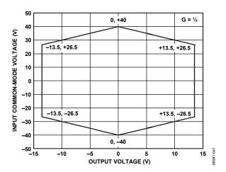
Figure 9. Input Common-Mode Voltage vs. Output Voltage, Gain = ½, ±15 V Supplies
