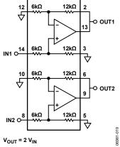
Figure 39. Noninverting Amplifier, G = 2
