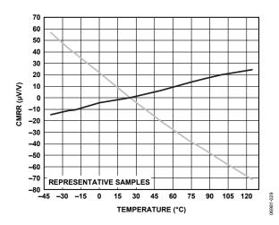
Figure 6. CMRR vs. Temperature, Normalized at 25°C
