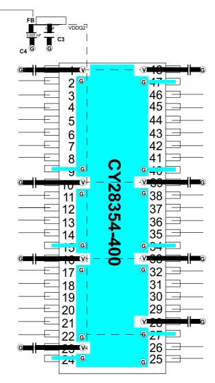
FB = Dale ILB1206 - 300 (300 $\Omega$  @ 100 MHz) or TDK ACB 2012L-120 Ceramic Caps C3 = 10–22  $\mu$ F C4 = 0.005  $\mu$ F
