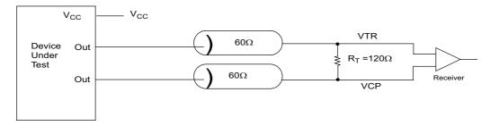
Figure 1. Differential Signal Using Direct Termination Resistor
