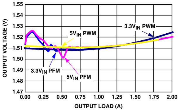
FIGURE 11.  $V_{OUT}$  REGULATION vs LOAD (1MHz,  $V_{OUT} = 1.5\text{V}$ )
