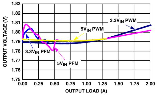
FIGURE 12.  $V_{OUT}$  REGULATION vs LOAD (1MHz,  $V_{OUT} = 1.8\text{V}$ )
