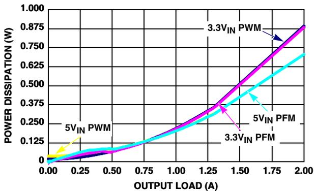
FIGURE 7. POWER DISSIPATION vs LOAD (1MHz,  $V_{OUT} = 1.8\text{V}$ )
