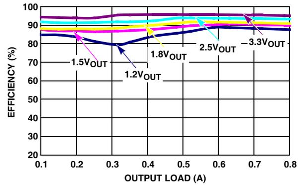
FIGURE 6. EFFICIENCY vs LOAD (1MHz 5VIN PFM)
