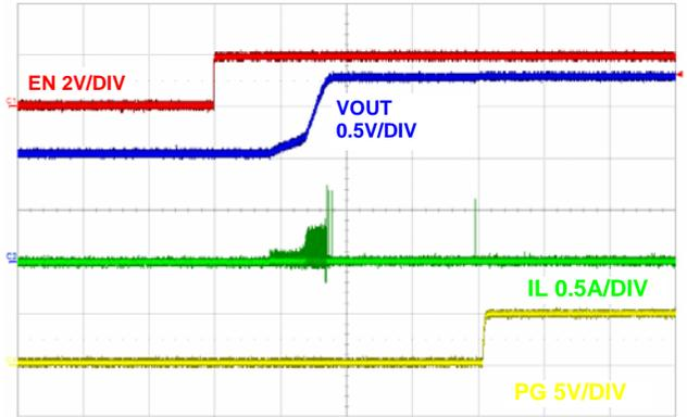
FIGURE 24. SOFT-START WITH PRE-BIASED 1V, (500 $\mu\text{s}$ /DIV)
