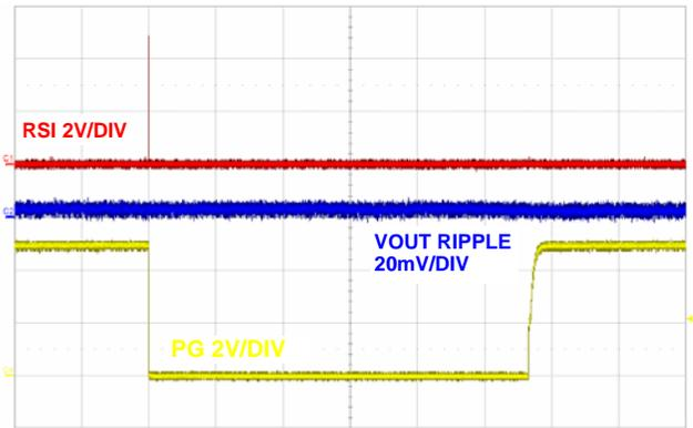
FIGURE 28. RSI RESET (ZOOM OUT), (200 $\mu\text{s}$ /DIV)
