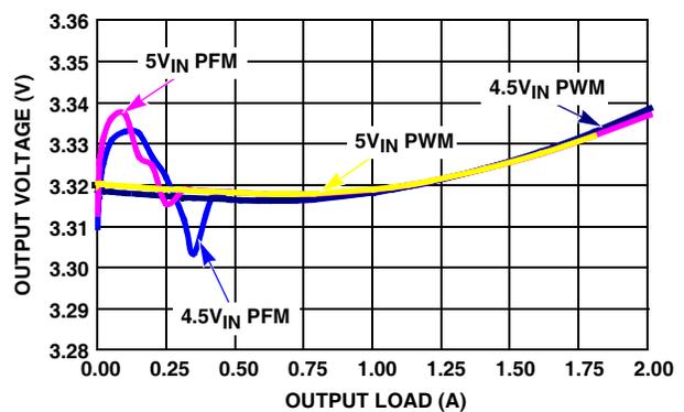
FIGURE 14.  $V_{OUT}$  REGULATION vs LOAD (1MHz,  $V_{OUT} = 3.3\text{V}$ )
