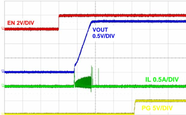
FIGURE 23. SOFT-START AT NO LOAD (PFM), (500 $\mu\text{s}$ /DIV)
