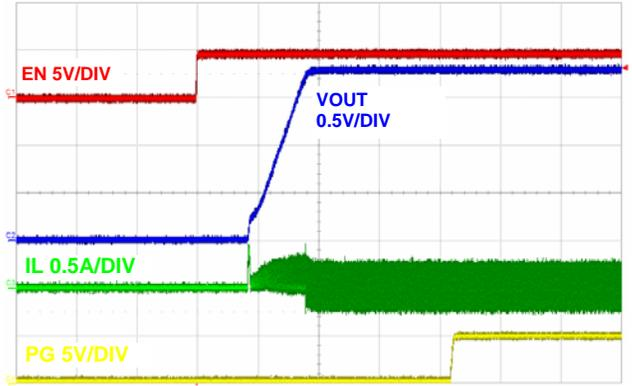
FIGURE 22. SOFT-START WITH NO LOAD (PWM), (500 $\mu\text{s}$ /DIV)
