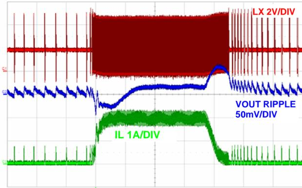
FIGURE 21. LOAD TRANSIENT (PFM), (500 $\mu\text{s}$ /DIV)
