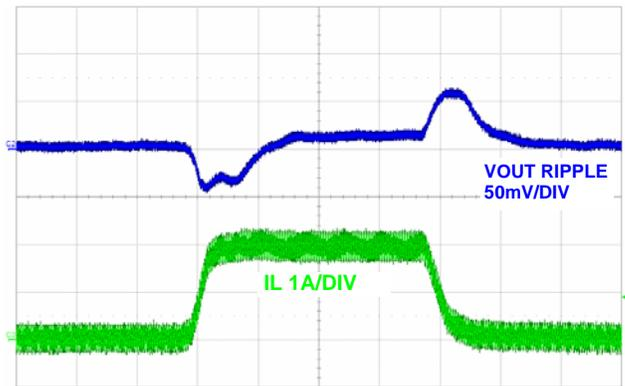
FIGURE 20. LOAD TRANSIENT (PWM), (50 $\mu\text{s}$ /DIV)
