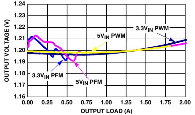
FIGURE 10.  $V_{OUT}$  REGULATION vs LOAD (1MHz,  $V_{OUT} = 1.2\text{V}$ )
