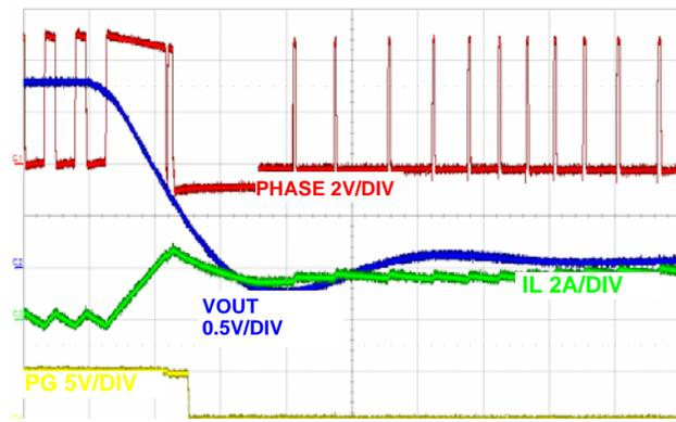
FIGURE 29. OUTPUT SHORT CIRCUIT, (500 $\mu\text{s}$ /DIV)
