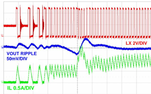
FIGURE 19. MODE TRANSITION DCM TO CCM, (50 $\mu\text{s}$ /DIV)
