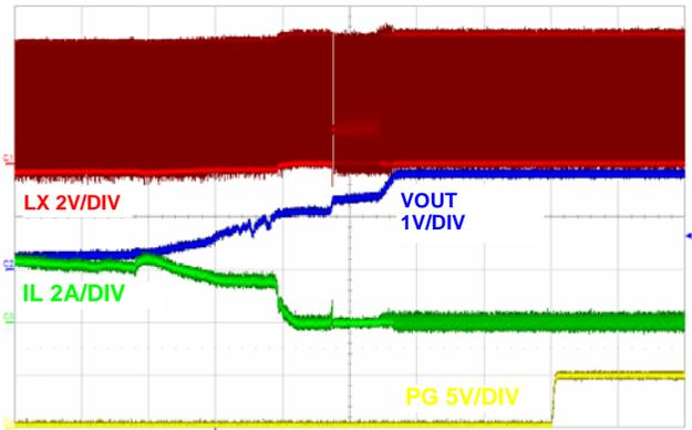
FIGURE 30. OUTPUT SHORT CIRCUIT RECOVERY, (500 $\mu\text{s}$ /DIV)
