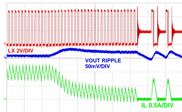
FIGURE 18. MODE TRANSITION CCM TO DCM, (5 $\mu\text{s}$ /DIV)
