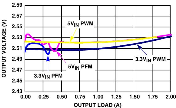
FIGURE 13.  $V_{OUT}$  REGULATION vs LOAD (1MHz,  $V_{OUT} = 2.5\text{V}$ )
