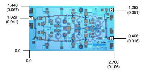
Units: millimeters (inches) Bond pad dimensions are shown to center of bond pad. Thickness: 0.110 +/- 0.010 (0.0043 +/- 0.0004), Backside is ground, Bond Pad/Backside Metallization: Gold All Bond Pads are 0.100 x 0.100 (0.004 x 0.004). Bond pad centers are approximately 0.109 (0.004) from the edge of the chip. Dicing tolerance: +/- 0.005 (+/- 0.0002). Approximate weight: 2.411 mg.
