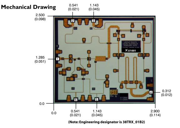
Units: millimeters (inches) Bond pad dimensions are shown to center of bond pad. Thickness: 0.110 +/- 0.010 (0.0043 +/- 0.0004), Backside is ground, Bond Pad/Backside Metallization: Gold All Bond Pads are 0.100 x 0.100 (0.004 x 0.004). Bond pad centers are approximately 0.109 (0.004) from the edge of the chip. Dicing tolerance: +/- 0.005 (+/- 0.0002). Approximate weight: 4.491 mg.
