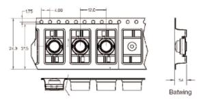
Figure 8. Tape dimensions for Batwing radiation pattern.
