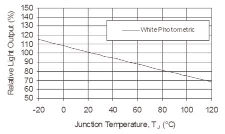
Figure 1. Relative Light Output vs. Junction Temperature.
