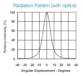
Figure 6. Typical Representative Spatial Radiation Pattern for LXHLNWG8.
