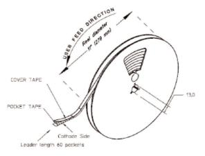
Figure 7. Reel dimensions and orientation.
