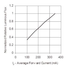
Figure 3b. Relative Luminous Flux vs. Forward Current at  $T_J = 25^{\circ}C$  Maintained.
