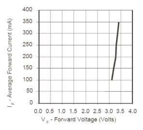
Figure 3a. Forward Current vs. Forward Voltage.
