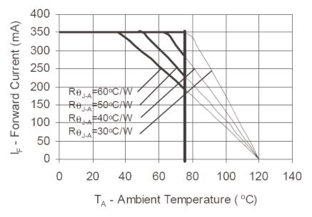
Figure 4b. Maximum Forward Current vs. Ambient Temperature. Derating based on  $T_{JMAX}$  = 120°C and  $T_{AMBIENT MAX}$  = 75°C for LXHLNWG8.
