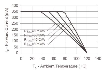
Figure 4a. Maximum Forward Current vs. Ambient Temperature. Derating based on  $T_{JMAX}$  = 120°C. Applicable for LXHLBW03 and LXHLMWGC.
