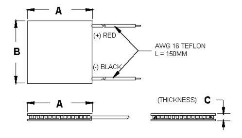
Ceramic Material: Alumina (Al<sub>2</sub>O<sub>3</sub>)
