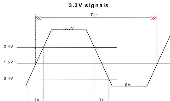
**Figure 7. Single-ended Output Signals (for AC Parameters Measurement)**
