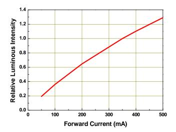
Forward Current Derating Curve, Derating based on  $T_{iMAX}$ =125°C
