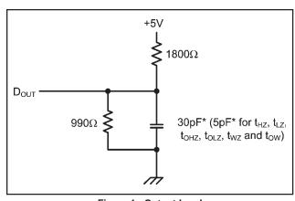
Figure 1. Output Load
