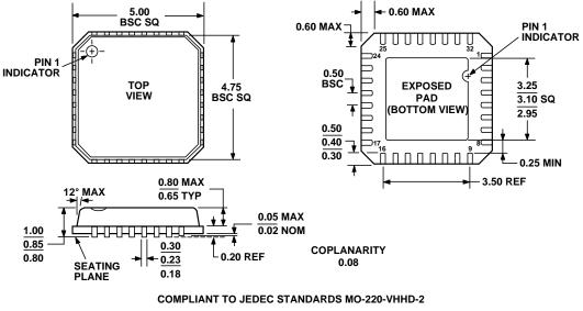
Figure 4. Mechanical Package Dimensions
