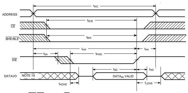
Write Cycle No. 4 ( $\overline{\rm BHE}/\overline{\rm BLE}$  Controlled,  $\overline{\rm OE}$  LOW)[18]
