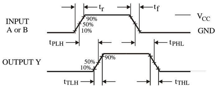
Figure 1. Switching Waveforms
