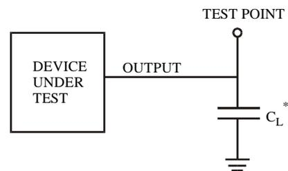
\* Includes all probe and jig capacitance
