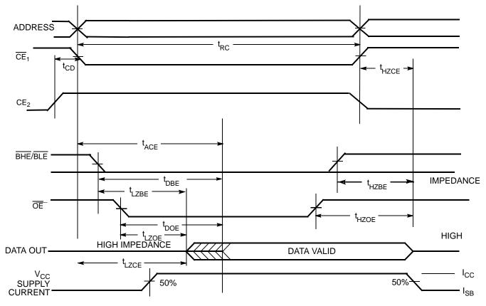
16. Whenever  $\overline{CE}_1$  = HIGH or  $\overline{CE}_2$  =  $\underline{LOW}$ ,  $\overline{BHE}/\overline{BLE}$  are taken inactive, they must remain inactive for a minimum of 5 ns. 17.  $\underline{\underline{Dev}}$  ice is continuously selected.  $\overline{OE}$  =  $\overline{CE}_1$  =  $V_{IL}$  and  $\overline{CE}_2$  =  $V_{IH}$ . 18.  $\underline{\underline{WE}}$  is HIGH for Read Cycle. 19.  $\overline{CE}$  is the Logical AND of  $\overline{CE}_1$  and  $\overline{CE}_2$ .
