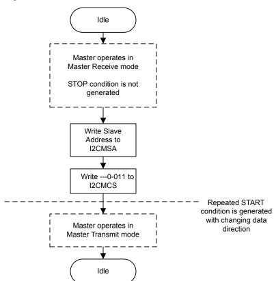
Figure 15-12. Master Burst SEND after Burst RECEIVE
