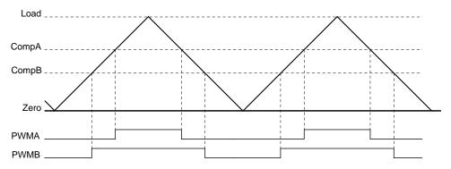
Figure 18-4. PWM Generation Example In Count-Up/Down Mode
