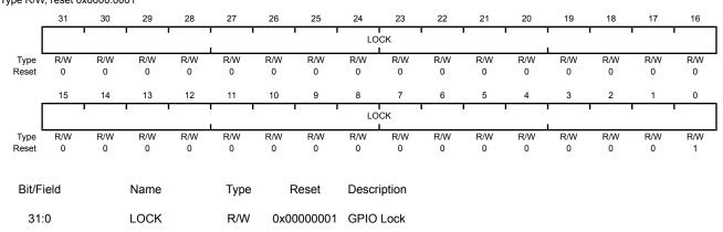
A write of the value 0x1ACCE551 unlocks the GPIO Commit register for write access. A write of any other value reapplies the lock, preventing any register updates. A read of this register returns the following values:
