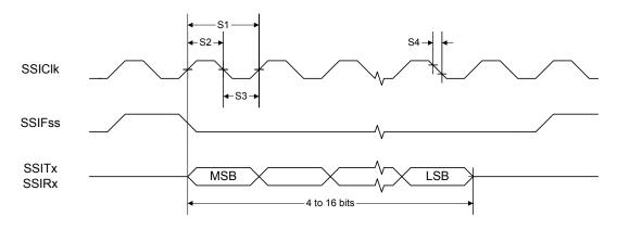
Figure 23-5. SSI Timing for MICROWIRE Frame Format (FRF=10), Single Transfer
