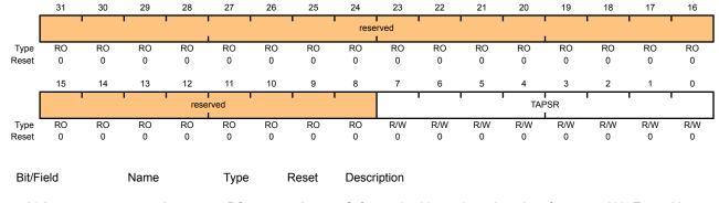
31:8 reserved RO 0 Software should not rely on the value of a reserved bit. To provide compatibility with future products, the value of a reserved bit should be preserved across a read-modify-write operation.
