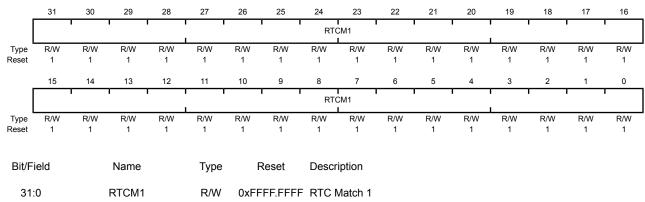
A write loads the value into the RTC match register.
