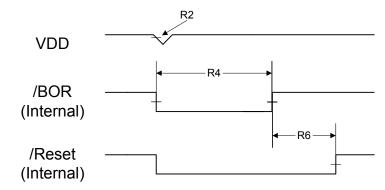
Figure 23-13. Software Reset Timing
