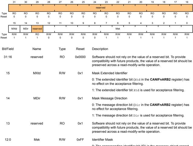
1: The corresponding identifier bit (ID) is used for acceptance filtering.
