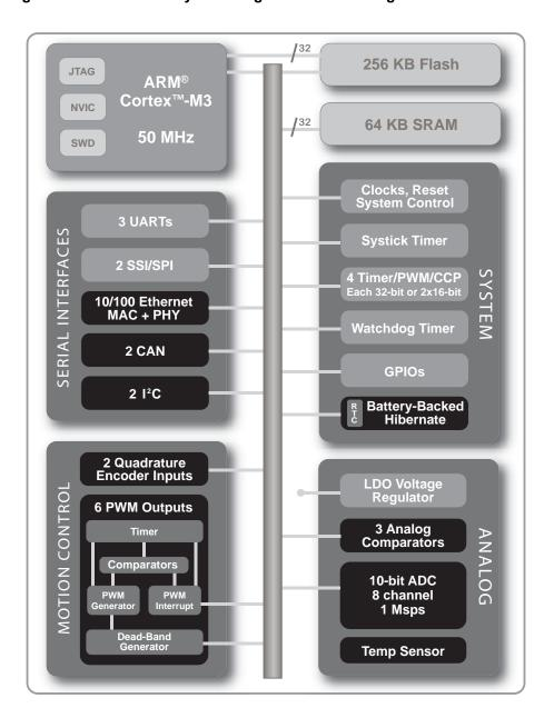
Figure 1-1. Stellaris® Fury-class High-Level Block Diagram
