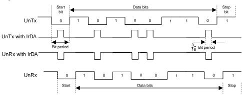
Figure 13-3. IrDA Data Modulation
