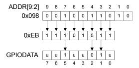
During a read, if the address bit associated with the data bit is set to 1, the value is read. If the address bit associated with the data bit is set to 0, it is read as a zero, regardless of its actual value. For example, reading address GPIODATA + 0x0C4 yields as shown in Figure 9-2 on page 156.
