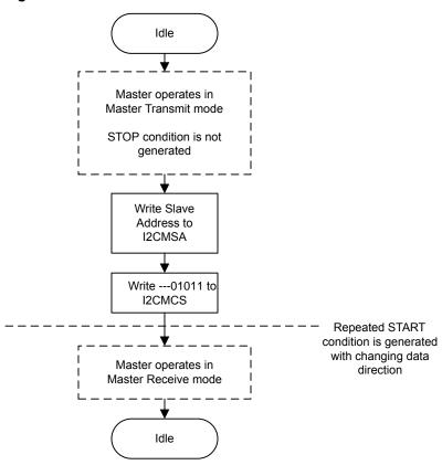
Figure 15-11. Master Burst RECEIVE after Burst SEND
