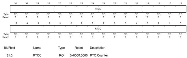
A read returns the 32-bit counter value. This register is read-only. To change the value, use the HIBRTCLD register.
