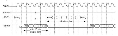
Figure 14-11. MICROWIRE Frame Format (Continuous Transfer)
