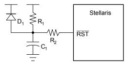
The  $R_1$  and  $C_1$  components define the power-on delay. The  $R_2$  resistor mitigates any leakage from the  $\overline{RST}$  input. The diode (D<sub>1</sub>) discharges  $C_1$  rapidly when the power supply is turned off.
