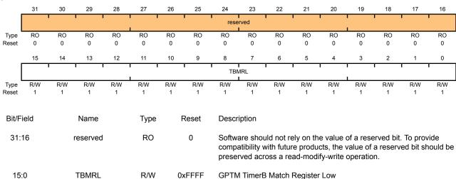
When configured for PWM mode, this value along with **GPTMTBILR**, determines the duty cycle of the output PWM signal.
