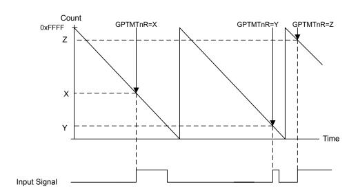
Figure 10-3. 16-Bit Input Edge Time Mode Example
