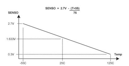
Figure 12-2. Internal Temperature Sensor Characteristic
