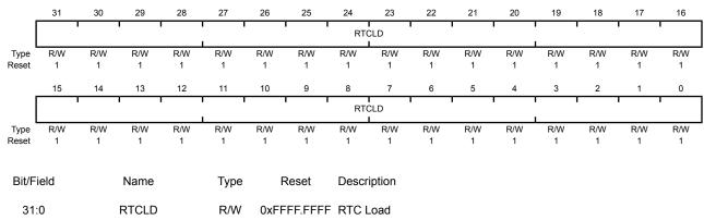
A writes load the current value into the RTC counter (RTCC).
