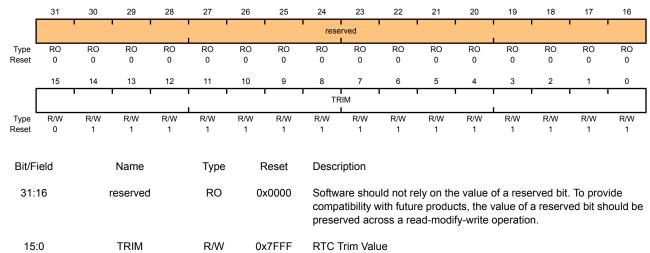
This value is loaded into the RTC predivider every 64 seconds. It is used to adjust the RTC rate to account for drift and inaccuracy in the clock source. The compensation is made by software by adjusting the default value of 0x7FFF up or down.
