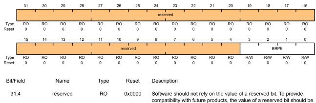
0x00-0x0F: Extend the BRP bit to values up to 1023. The actual interpretation by the hardware is one more than the value programmed by BRPE (MSBs) and BRP (LSBs) are used.
