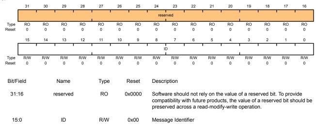
This bit field is used with the ID field in the **CANIFnARB2** register to create the message identifier. ID[28:0] is the Extended Frame and ID[28:18] is the Standard Frame.
