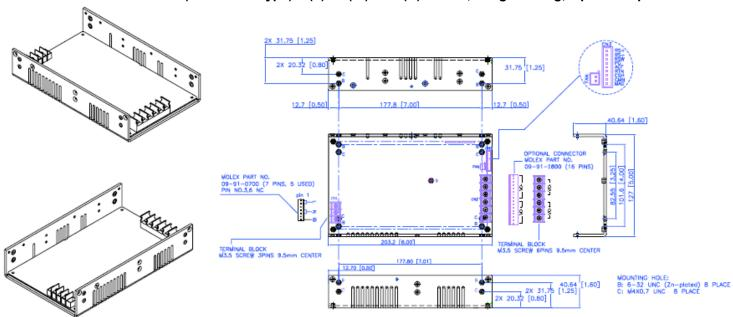
PSRL0402E-I Series (Enclosed with built-in Fan Type): 9(L) x 5(W) x 1.6(H) inches; Weight: 1.6kg.
